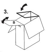
Bring down the wire to the other side of the box and fold over flap B. Check to make sure that the wire is at the top of the box tucked under the flaps.
